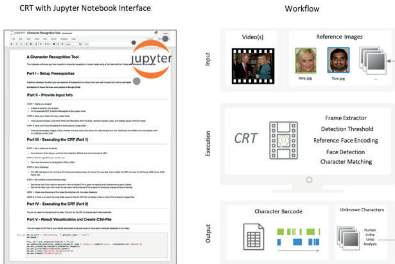
Figure 2 CRT User Interface and Principle
